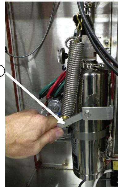
Insert the shipping pin (6) into the valve handle (14). Move the spring lever (1) up to relieve tension on the s-hook and valve handle.
