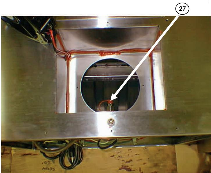
With the fan removed the plenum nozzle is exposed (27). Inspect the nozzle and blow off cap.
